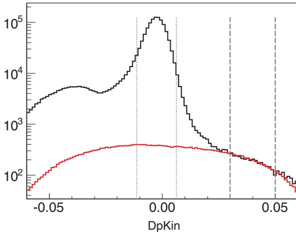
FIG. 2. (Color online) The  $DpKin$  distribution for the hydrogen target (thick black histogram) and the dummy targets (thin red histogram). The dashed vertical lines indicate the region used to normalize the dummy contribution to match the contribution from the aluminum end caps of the hydrogen target and the vertical dotted lines indicate the part of the elastic peak used in the analysis.
